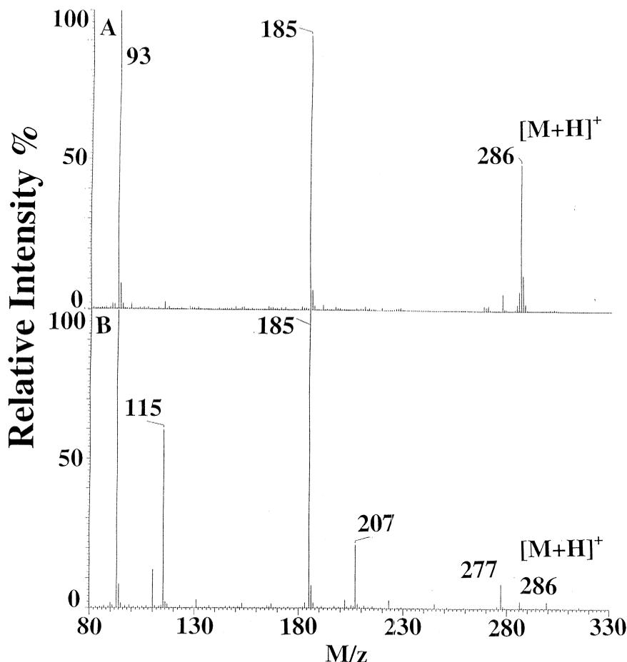
Fig. 1. The double focusing HPTLC–FABMS spectra obtained directly from the silica gel of the HPTLC plate for (A) a spot for a pure standard of morphine and (B) a spot corresponding to morphine obtained from HPTLC of a urine extract.
