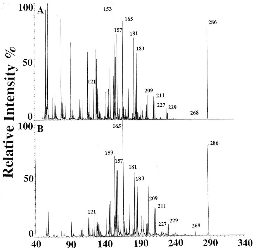
Fig. 2. The HPTLC–FABMS–MS spectra obtained from the ion at  $m/z$  286 for (A) the spot of the pure standard of morphine shown in Fig. 1A and B the spot corresponding to morphine seen on the HPTLC of a urine extract and shown in Fig. 1B. The proposed fragmentation map is shown in Fig. 3.
